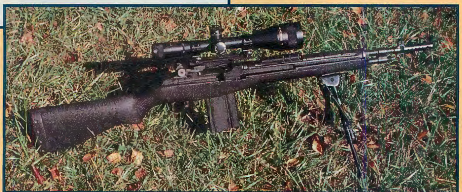
Rather than a flash suppressor the M1A Scout Rifle has an extremely efficient muzzle brake (above) that cuts muzzle jump down to almost nothing with most loads. (right) M1A Scout rifle with a 10X Springfield Mil-Dot Government Model scope and mount with a Harris bipod. This rig could be used as a military or police sniper rifle or as a long range hunting rifle.
