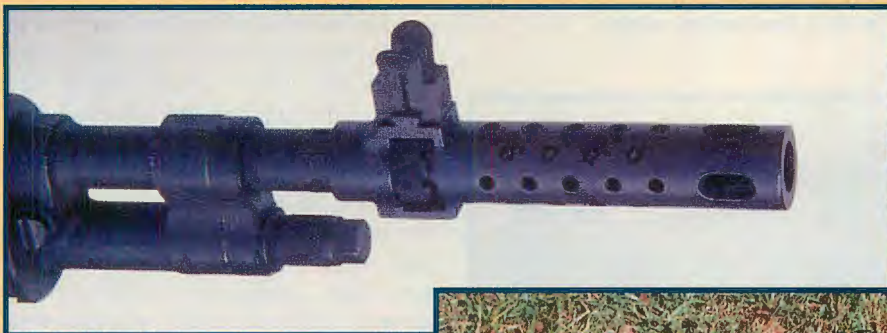
Rather than a flash suppressor the M1A Scout Rifle has an extremely efficient muzzle brake (above) that cuts muzzle jump down to almost nothing with most loads. (right) M1A Scout rifle with a 10X Springfield Mil-Dot Government Model scope and mount with a Harris bipod. This rig could be used as a military or police sniper rifle or as a long range hunting rifle.
